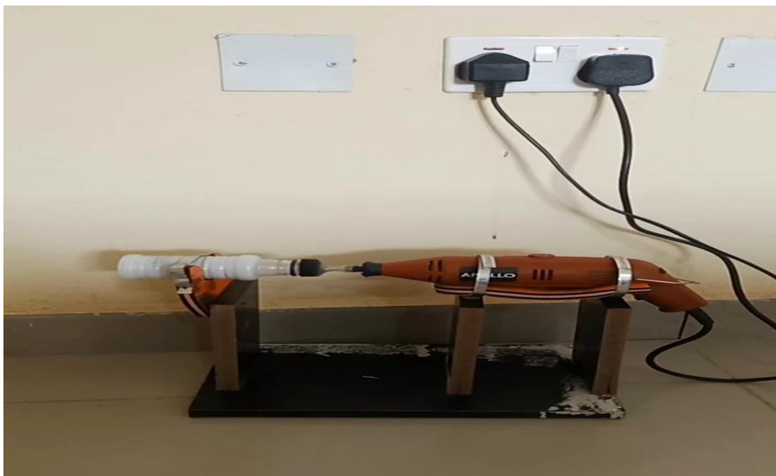
Figure 4. Gyrotory Induced Adhesive Coating Method
