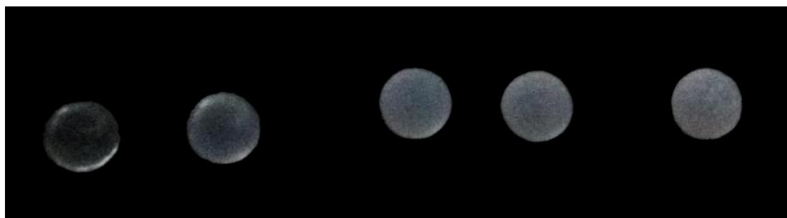
Figure 2. Glass beads coated using the GIAC method. Left to right: loadings of 0, 1, 3, 5 and 7
